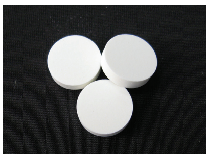
Linseed oil tablet, Ø11.3mm, 125N at 500kg/cm 2
